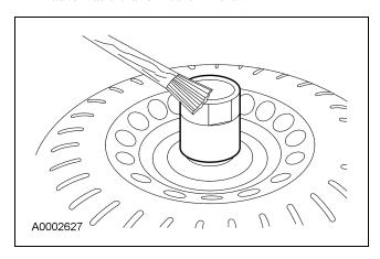
Using the special tools, install the torque converter by pushing and rotating.
